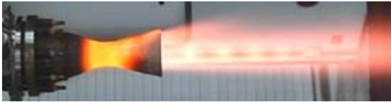
Fig 16: Sea level testing of ceramic engine
