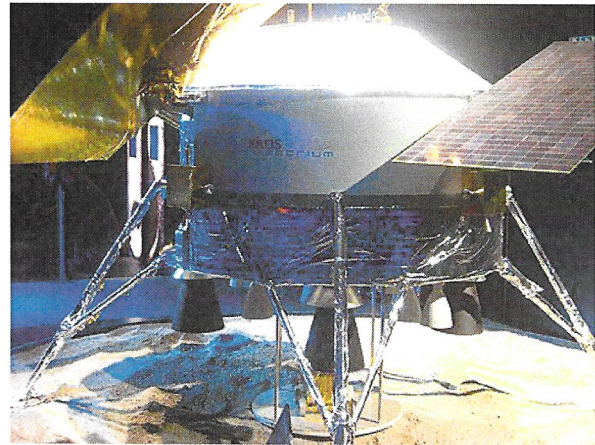
Figure 10: Astrium proposal for a Lunar Lander Module concept with 220 N and 500 N Engines (mock-up model).
