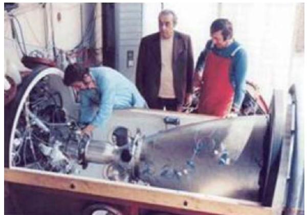
Fig. 2. Integration of the HM7 Engine with NE in the vacuum capsule with thrust measurement rig.
