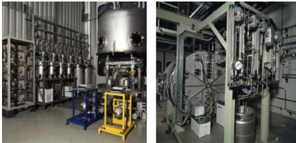
Fig. 20. Test facility test cells for satellite propulsion thrusters.
