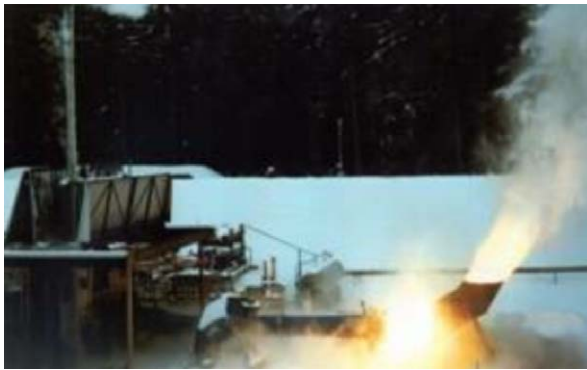
Fig. 3. Test of the HM7 B third stage thrust chamber under altitude conditions.
