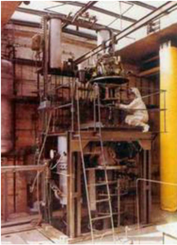
Fig. 9. P 1.5 high altitude test facility up to 400N.
