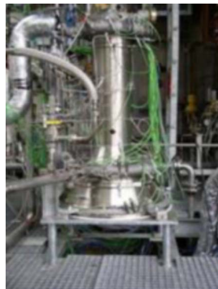
Fig. 25. Test set-up of Vinci CC for LH2 Flow tests.
