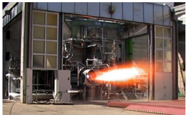
Fig. 29. Hot firing of the Vinci thrust chamber.
