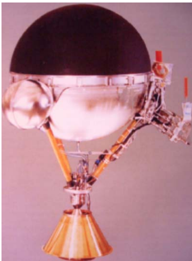
Fig. 10. Apogee boost system for Symphonie.
