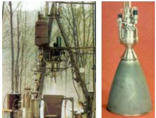
Fig. 7. Sea-level tests of the 400N engine as well as the 400N engine with regenerative cooled throat-area.
